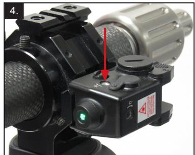
Use the horizontal set screw to adjust the laser, left or right.
