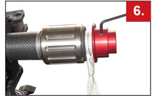
Push retainer tightly against the loop and torque down the Set Screw securely. Screw will indent into the Breech Plug, slightly.
