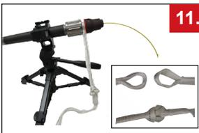
Connect Lanyard to Parachute as shown.
